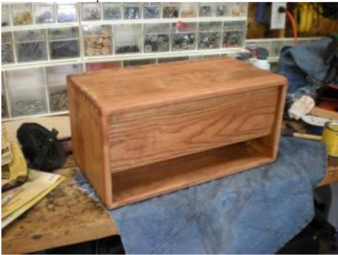
Now you can rout all the inner edges of the front and back edges with your round-off bit.
