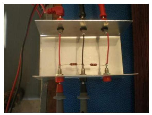
You'll need a 1-ohm resistor for each power tube in the amp. The EL-34 tubes have their cathodes on pin EIGHT, which will be grounded to the chassis. Pin ONE will be tied to pin EIGHT, and both will be grounded- you will need to untie them before proceeding with this method.
