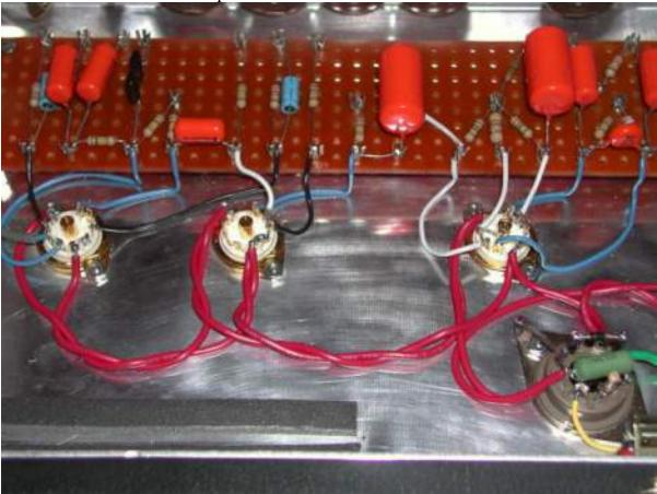
PVC-coated solid-core 20 AWG wire was used in the original Expresses and the same wire is used in this amp. The color code, wire length and proper wire specifications correspond exactly to the layout found in Francesca. Shielded wire was used from the input jack to the input of the first preamp stage. This is the only shielded wire in the amp.
