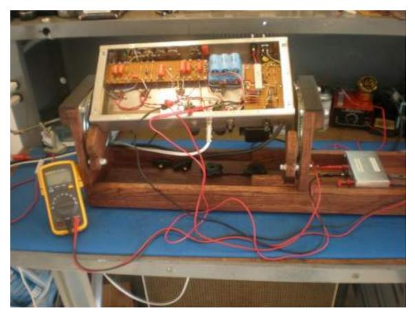
Turn your amp on, but leave it on STANDBY. Set your DMM to the highest DCV scale, ground the black probe to the chassis, and take a reading from pin FIVE of any power tube socket. You should see a negative voltage in the -35 to -50 volt range for EL34s. Note that you should \*not\* have any power tubes installed in your amp yet.
