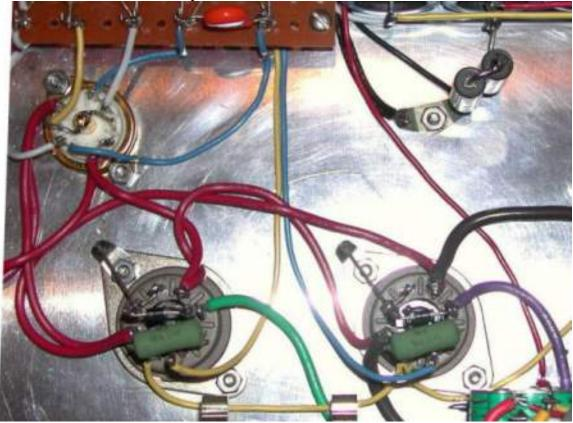
The phase inverter (at upper left in the picture above) is a 12AX7 long tail phase inverter, not unlike those used in Fender and Marshall amplifiers. It is sometimes referred to as the "driver tube" because it supplies two output signals 180 degrees out of phase to drive the two power tubes.
