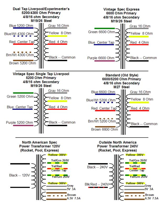
Yellow 300v secondary wires - to diode stack on PS board Yellow/Green 260v secondary wires - not used Yellow/Red 0v - to ground lug under power cord Gray 5v - not used (clip short and heat shrink) Brown 6.3v - heaters Brown/White center tap - to ground lug under power cord
