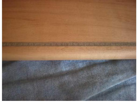
I routed a 1/4" radius on the outer edges and corners using a round over bit. Don't do the inner edges until you are done measuring for the chassis bolt holes installing the front panel- you want a straight edge to work with.
